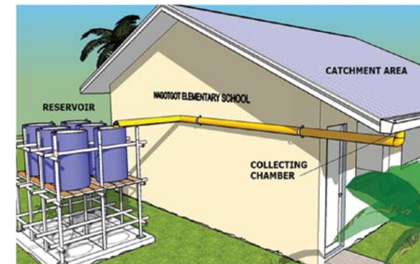
THE SOLUTION – A RAINWATER RESERVOIR
